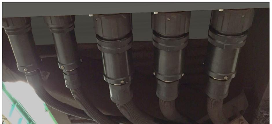
The fully assembled cable junction box on the underside of the car with the GIMOTA sliding backshell and the PMA screw connections.
